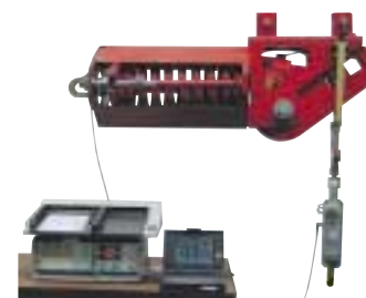
Testing constant hangers on site with a mobile test bench.
